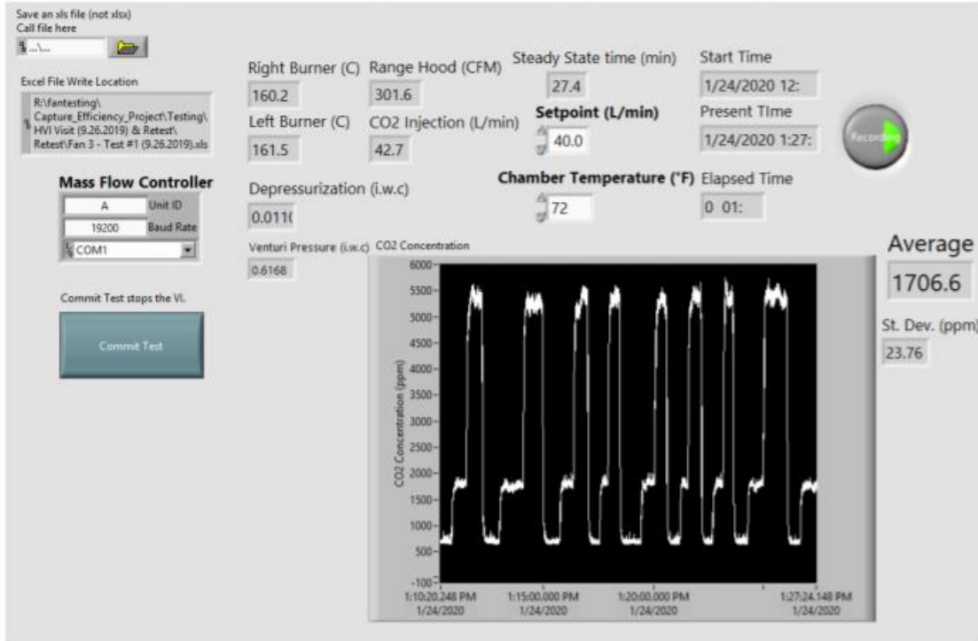
Figure 9: LabVIEW Software Used to Take CO 2 Measurements
