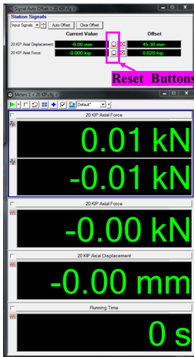
Figure 3.21 Real-time force-displacement-run time meters on the MTS Station Manager software
