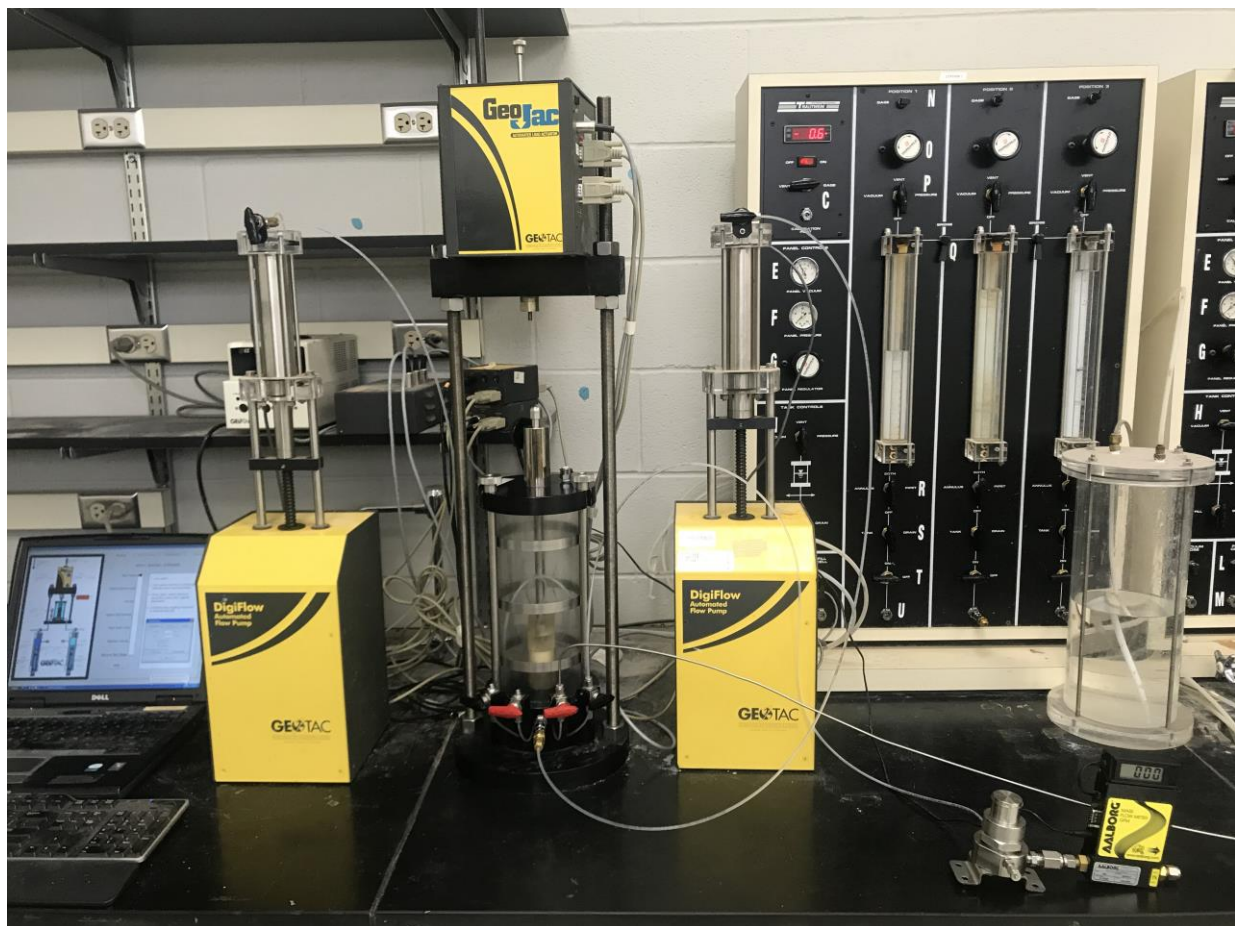
Figure 4.24 Setup for gas permeability tests with triaxial cell
