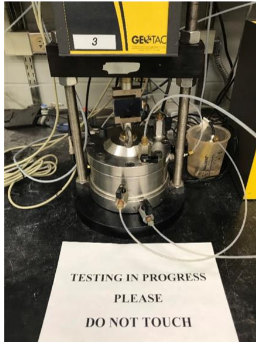
Figure 4.10 Setup for swelling pressure measurements
