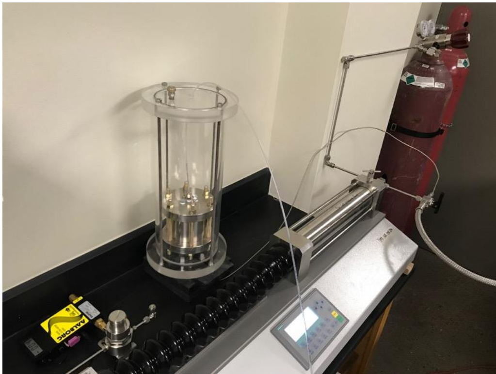
Figure 4.30 Setup for gas breakthrough tests
