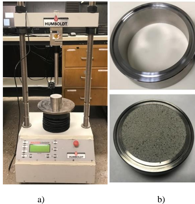
Figure 4.36 Load frame for compaction and mold
