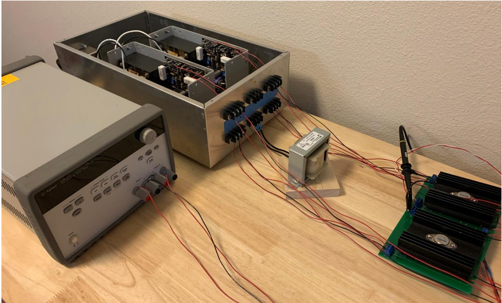
Figure 4.3: Power supply arrangement. The open enclosure contains both of the fixed, linear power supplies used for the transconductance amplifier. The programmable power supply is used to power the modified Pierce oscillator.
