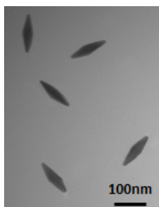
Figure 10. TEM image of AuNBPs-PA-IgG following storage at 60^\circ\text{C} for 48 hours.
