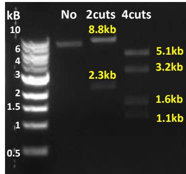
Figure 5.6. Results of restriction enzyme digestion of plasmid pTipQC2-Up-dypB-Gen-Down. The plasmid (pTipQC2-Up-dypB-Gen-Down) was digested with HindIII and BamHI (2 cuts, expected size: 8.8 and 2.3 kb), XbaI and XhoI (4 cuts, expected sizes: 5.1, 3.2, 1.6 and 1.1 kb), or without enzymes (No: no restriction digestion, 8.0 kb).
