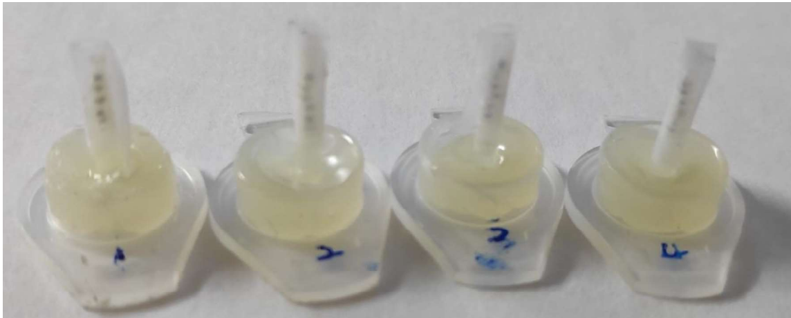
Figure III.3. The configuration to examine the morphology of Ni-P coatings deposited on diamond abrasives.
