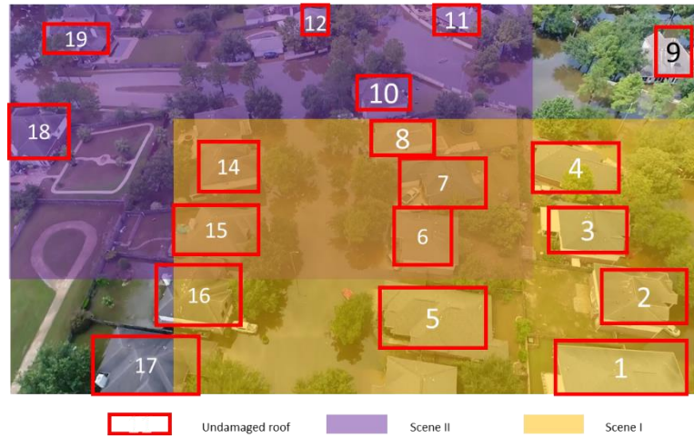
Figure 54. Reference points updating for homography transformation.
