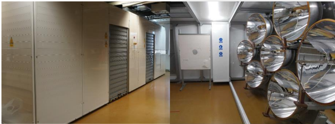
Figure 4: Outside and inside view of the new ultra high flux solar simulator (UHFSS) facility at TAMUQ.
