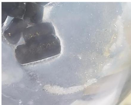
**Figure 42.** Phosphoric acid-modified Norit<sup>®</sup> pellets during the desorption experiment.
