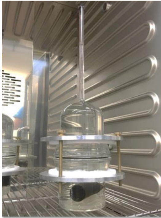
Figure 19. Amott Cell placed in the oven at the reservoir temperature.
