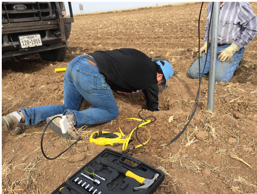
Figure 3.6: Deploy soil moisture sensors in the field.
