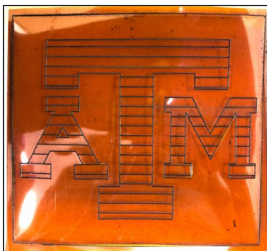
Figure 3-1. A 76.2 mm x 76.2 mm sample of Kapton that has been etched by a CO 2 laser (30% laser power, 50% etch speed, 1000 PPI). The pattern displayed was designed prior to lasing using AutoCAD.
