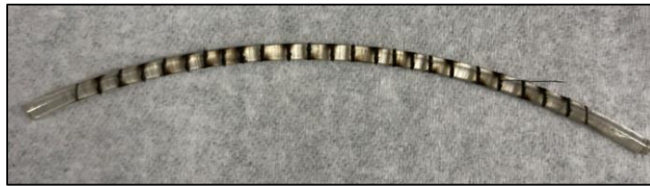
Figure 2-6. A prototype LIG@PESU printing filament developed at TAMU (5% laser power, 10% etch speed, 1000 PPI). Filament diameter is 1.75 mm, typical for material extrusion 3D printers.
