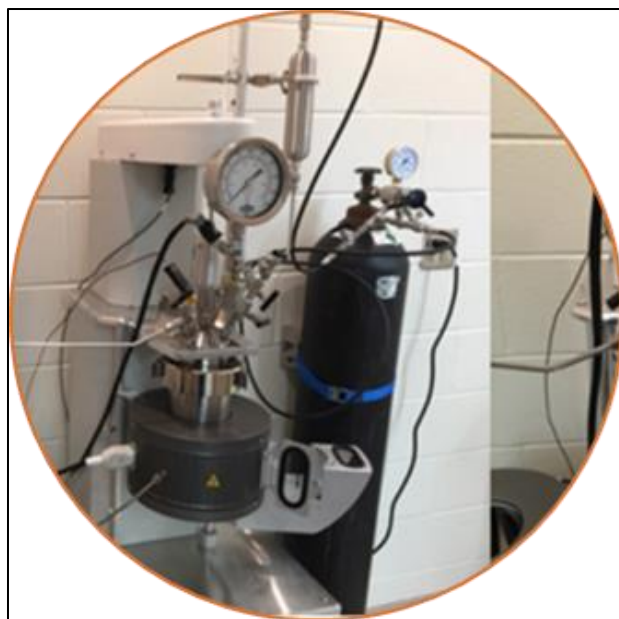
Figure 25-a Parr 4520 bench top reactor.
