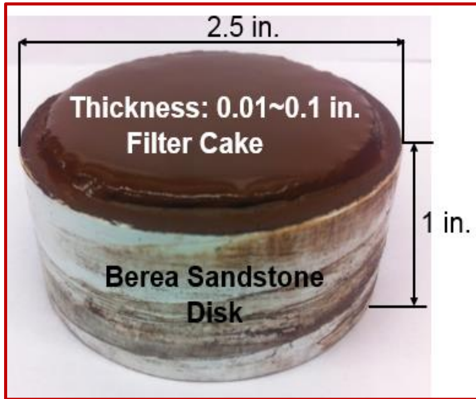
Figure 18 Berea sandstone disks with filter cake formation. Reprinted with permission from SPE-190115-MS.
