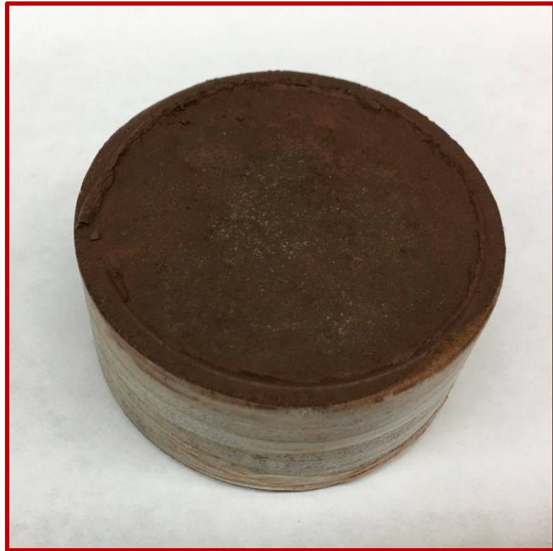
Figure 19 Berea sandstone disks after filter cake removal. Reprinted with permission from SPE-190115-MS.
