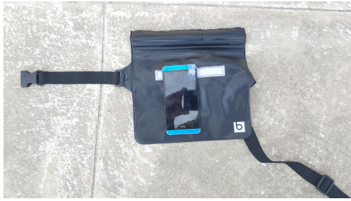
(a) Initial prototype design, involving a waterproof pack, an HTC Android phone, and harness (b) Initial prototype design being worn by a swimmer
