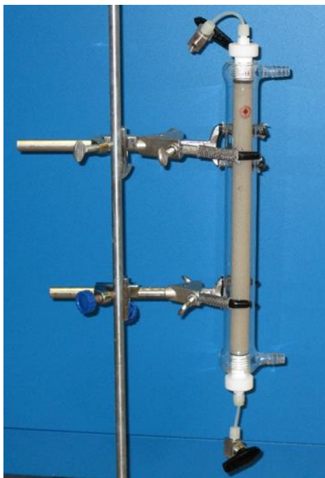
Figure 27: Sandpack Glass Chromatography Column, PTFE Endcaps, Nylotube, and Swagelok Three-Way Valves
