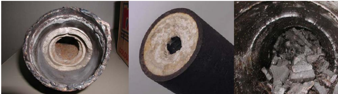
Figure 4: Typical Oilfield Scales (Mackey, 2007) – (Left & Center) Scale and other debris formation along sides of pipe. (Right) Suspended particles in plug formation and filtration equipment.
