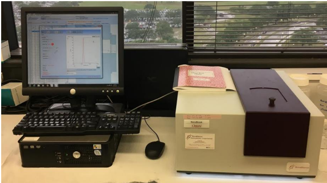
Figure 10: NanoBrook Omni Particle Sizer and Zeta Potential Analyzer by Brookhaven Instruments Corporation
