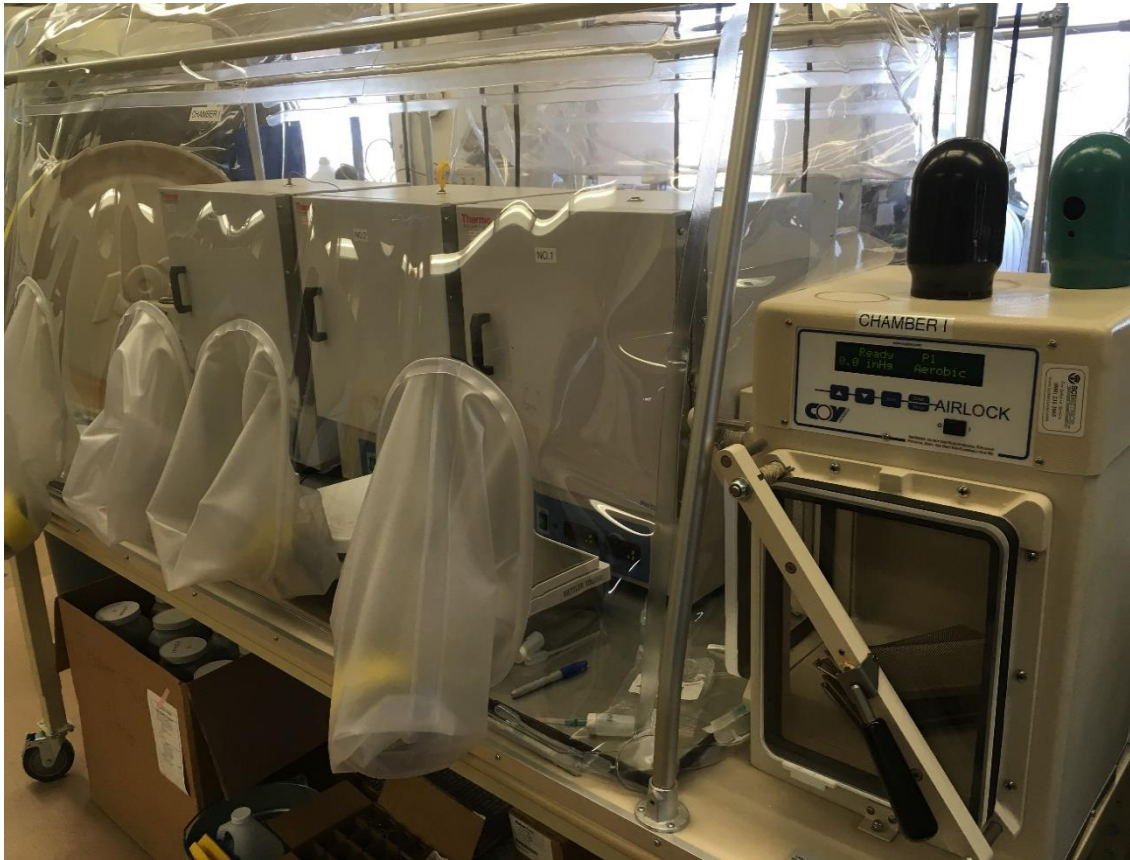
Figure 8: Anaerobic Chamber Containing a Stirring Plate, Mass Balance, High Temperature Ovens, Condensation Catalyst, Circulation Fan, and H 2 /O 2 Detector
