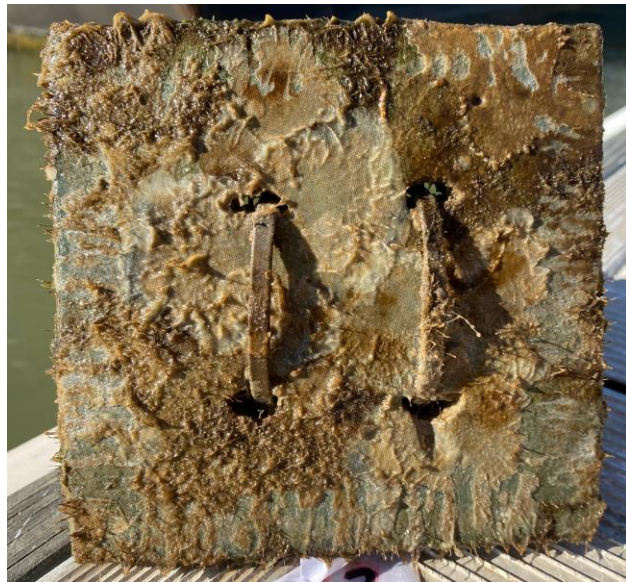
Figure 2: Notice the repeated scrape marks around the perimeter of this CM2 panel at 8 weeks. This same pattern was seen on multiple other CM1 and CM2 panels. The fibrous organisms, which appear to be hydroids along the left upper edge and around the lower left hole, fell below 1% cover before the end of deployment. Hydroid populations decreased on all panels after 10 weeks.
