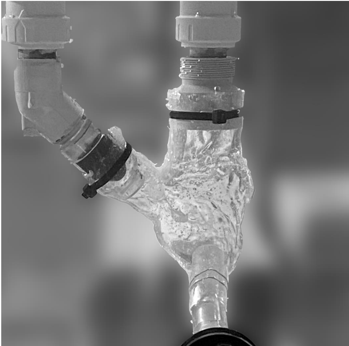
Figure 3-4: The Optically Clear Deformable Sac – The optically-clear silicone ventricular sac features dense trabeculations specific to the HLHS patient.
