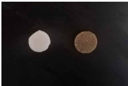
Figure 3: A non-coated sample (left, 6 x 2 mm) and coated sample (right, 6 x 2 mm).
