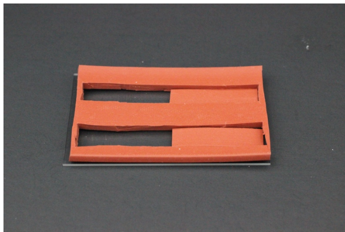
Figure 4: Interfacial Lap Shear Testing Custom Mold
