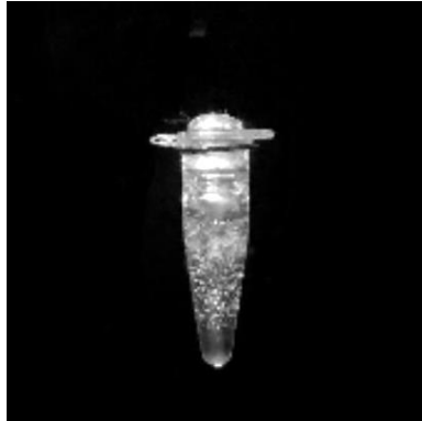
Figure 18: 3D Reconstruction of the vial of gelatin from the first OCT simplification
