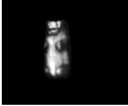
Figure 35: 3D Reconstruction of the red gummy bear from the third OCT simplification
