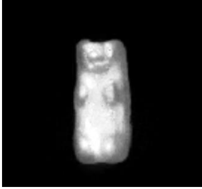
Figure 15: 3D Reconstruction of the red gummy bear from the first OCT simplification
