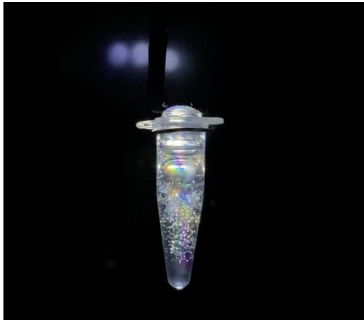
Figure 4: Still of the vial of gelatin with air bubbles added before solidification from the initial OCT simplification
