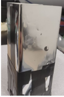
(a) Scintillator crystal wrapped with Aluminized PET material after the first layer of reflective material. This PET material was to reflect background light noise away from the scintillator.
