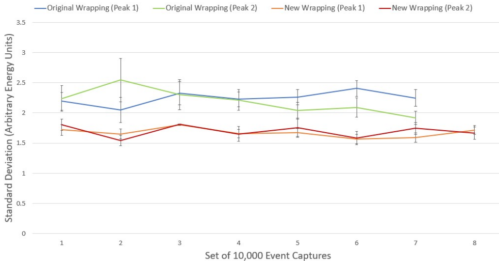
Figure 8: ^{60}\text{Co} systemic check for drifting over time. Plot of the standard deviation with uncertainty in arbitrary energy units of each set of 10,000 events for both peaks for the original (shown in blue and green) and new ESR wrapping (shown in orange and red).
