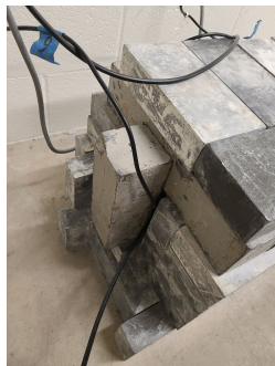
(a) Front of the lead structure displaying the small, necessary opening where the wires can come out to connect to the rest of the hardware. The scintillator detector is placed completely in this lead structure.
