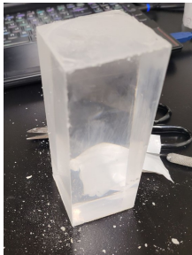
(a) Unwrapped 6 inch CsI(Tl) crystal. The crystal is very clear, free from impurities, and major chips or scratches.
