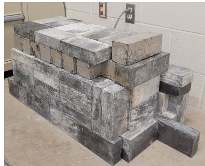
(b) Full view of the lead structure from behind. Each wall on the lead structure, except for the small opening for the wires, is 6 inches thick. This is to reduce high energy background noise like cosmic rays.
