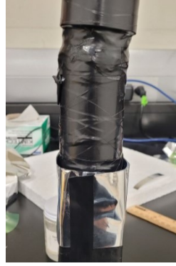
(c) Aluminized PET material around the connection point between the PMT photocathode and the crystal to prevent background noise coming in at the connection point.
