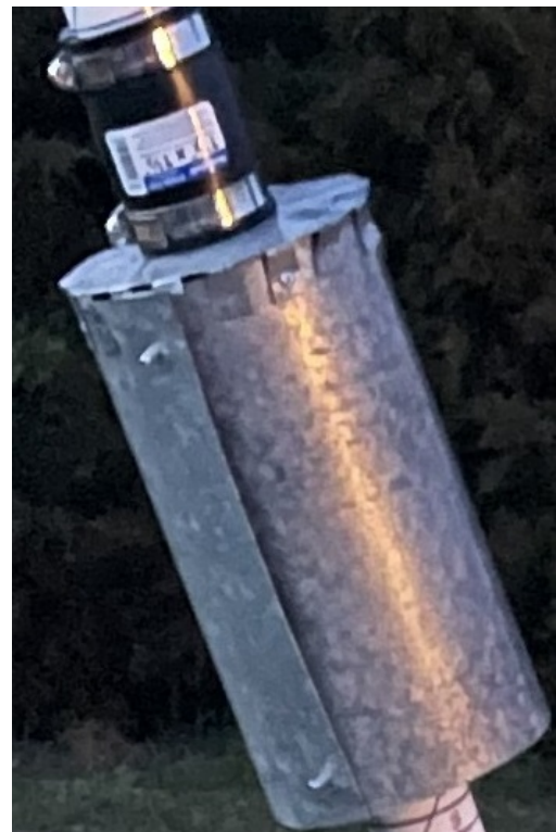
Figure 12: Parts to assemble waveguide and final waveguide.
