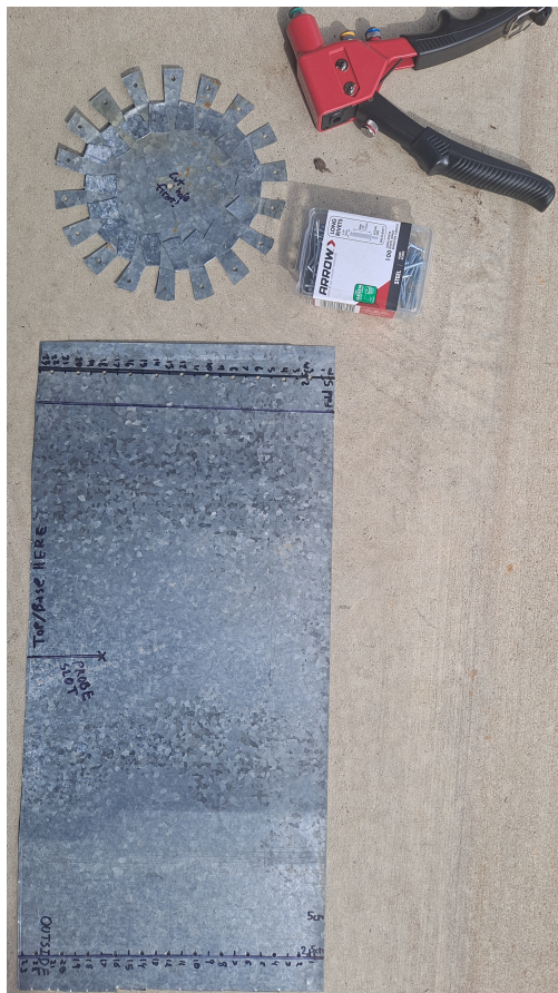
Figure 12: Parts to assemble waveguide and final waveguide.
