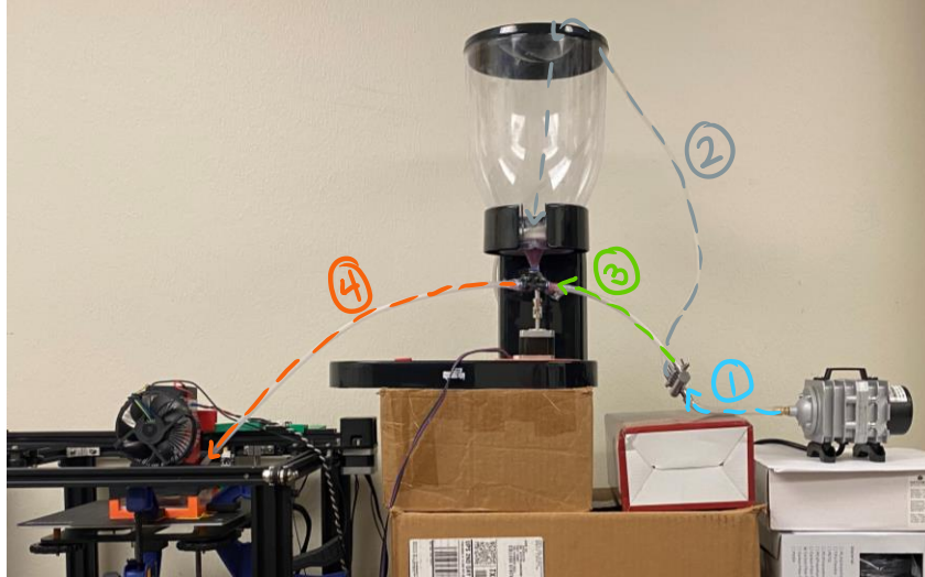
Figure 4: Air flow path of system
