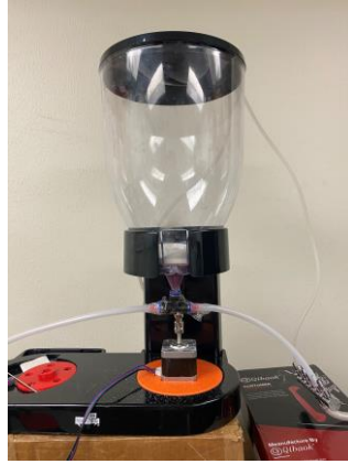
Figure 5: Reservoir with rotating powder feeding mechanism and powder
