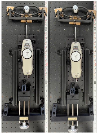
Figure 5.12: Bi-stable Mechanism Gripping Force Experiment.
