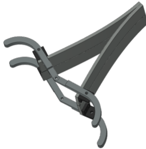
Figure 2.2: Strong Jaw Gripper Design Concept.
