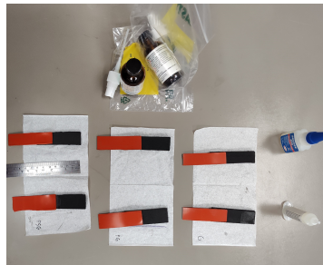
Figure 3.17: Creating samples of various adhesion methods between the SL and SRL materials
