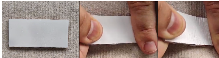
Figure 3.12: The paint experiences plastic strain after one full cycle.
