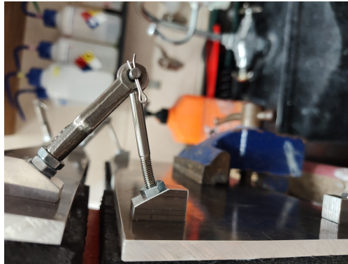
Figure 3.3: The first prototype placed on the panel system was enough to bend the hinges.
