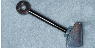
Figure 1.7: The hinge pin (c.f. 1.4) is connected to the base with a rod-shaped hinge leaf.
