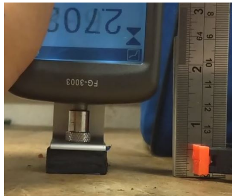
Figure 3.16: Compression test setup and example
