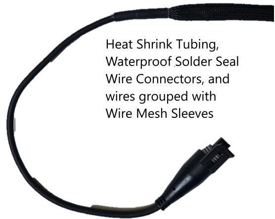
(b) Wiring Harness Improvements
