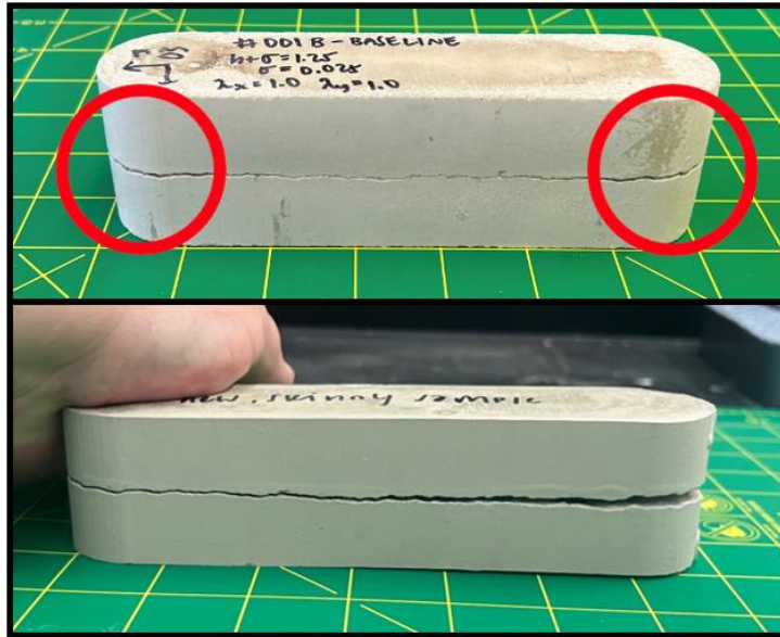
Figure 60: Illustration of the Divergence of Matching Surfaces on Sample Flanks
