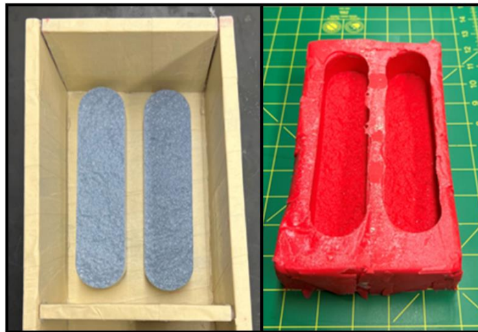
Figure 28: Conductivity Cell Fracture Sample Casting (Reprinted from Sistrunk et al. 2023)
