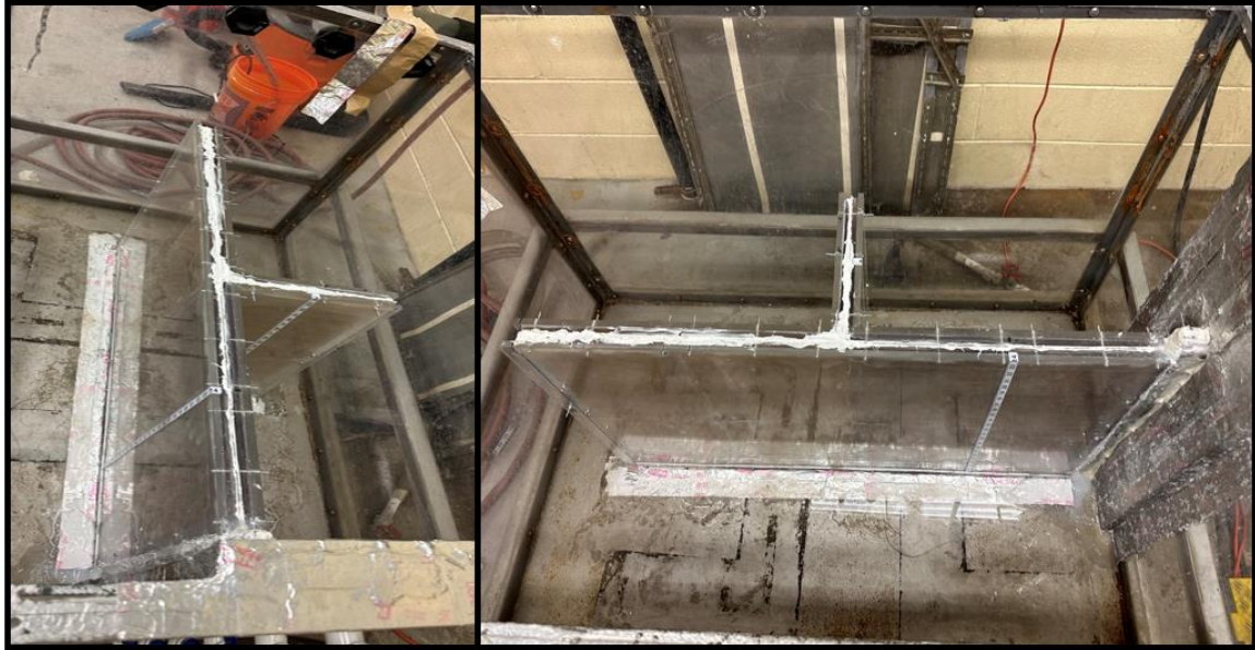
Figure 58: Post-Assembly Proppant Transport Experimental Apparatus
