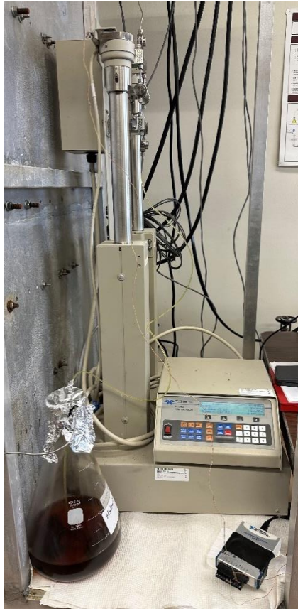
Figure 7 – Teledyne ISCO syringe pump and hydraulic oil reservoir flask
