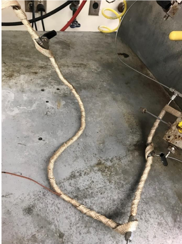
Figure 11 – Heating tape wrapped around the tubing to heat up the fluid
