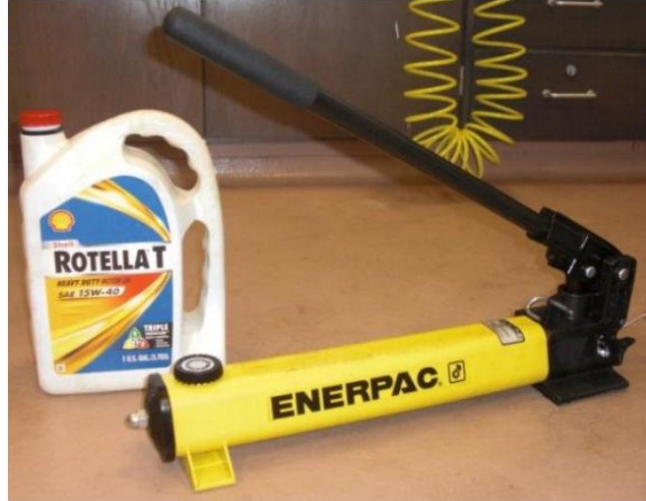
Figure 6 – ENERPAC-392 hydraulic hand pump (Grabski, 2012)
