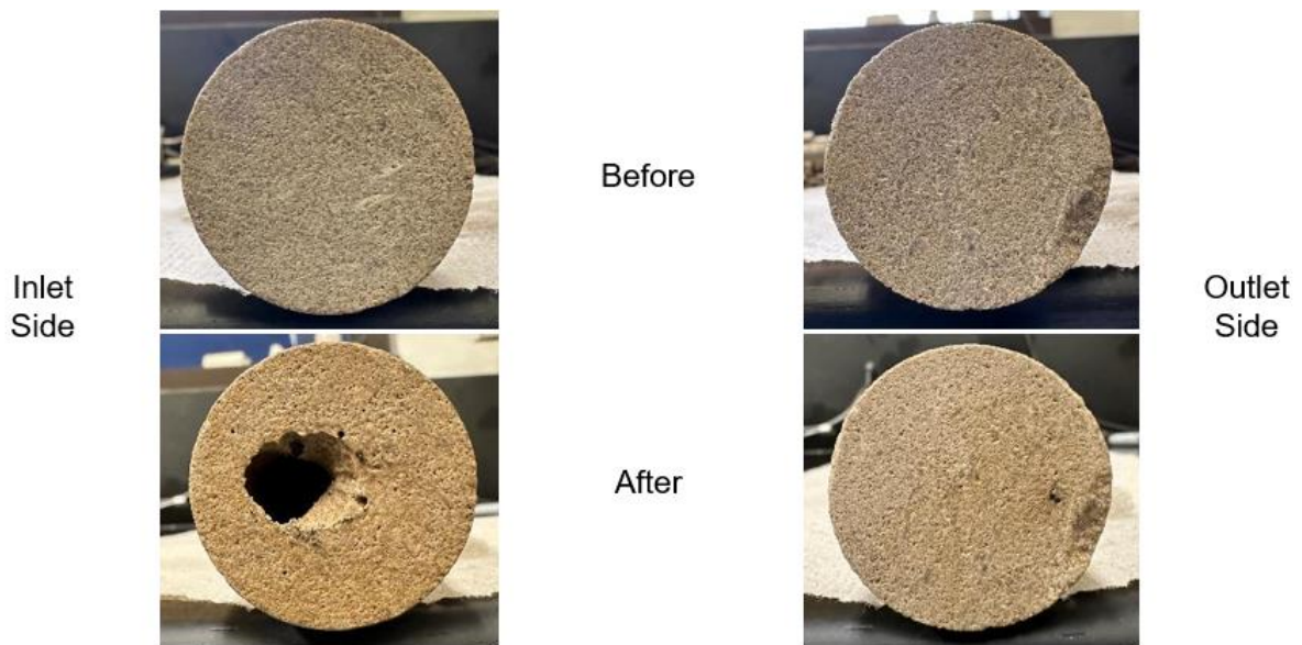
Figure A20 – Core H-225-2 (Injection rate = 4.5 mL/min at 225°F)
