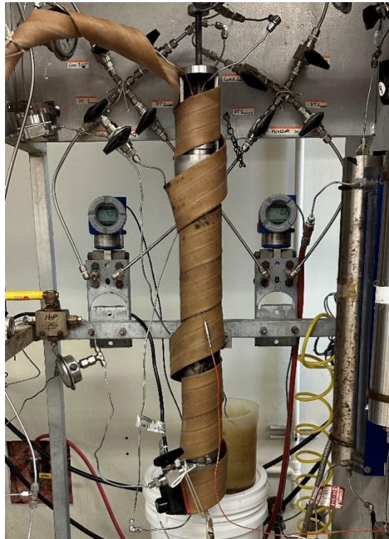
Figure 10 – Core holder with heating tape
