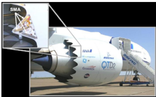
(a) SMA Chevrons on Engine Outlet[17]
