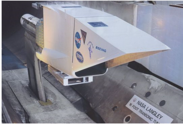
(a) SMA Embedded F-15 Inlet
