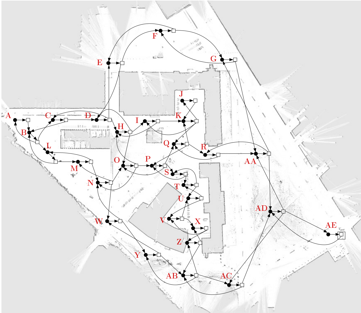
Figure 3.2: The example world from Figure 3.1 as a p-graph with goal region. Here, we consider every observation vertex (filled circle) to be a possible initial configuration. Observation vertices give distinct observations as output, while the actions include movement in the cardinal and intercardinal directions. Labels showing these have been omitted for clarity of the figure.
