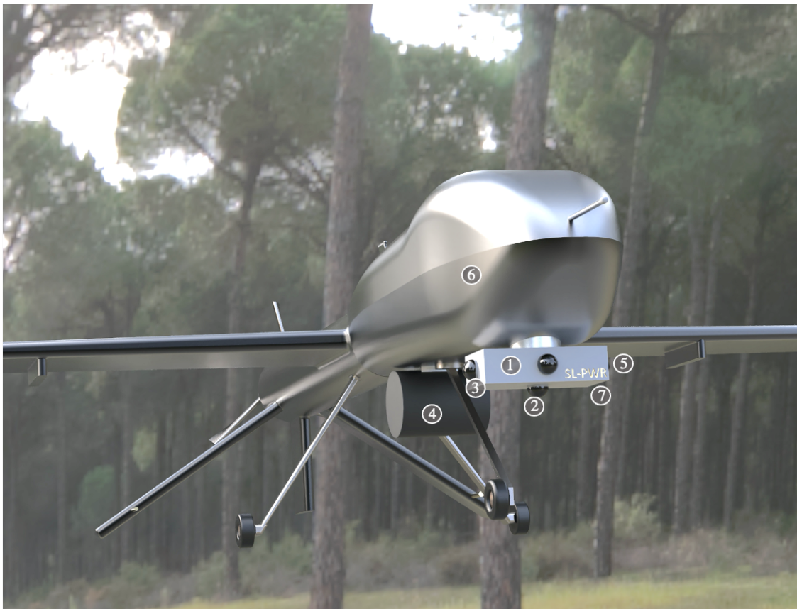
Figure 7.2: The SL-PWR Prototype Deployment. 1.) Controller and Software BrainBox, 2.) Main View Camera, 3.) Lateral View Cameras 4.) SL-PWR Fluid Holder, 5.) Thermal sensor, 6.) UAV, 7.) Communication module
