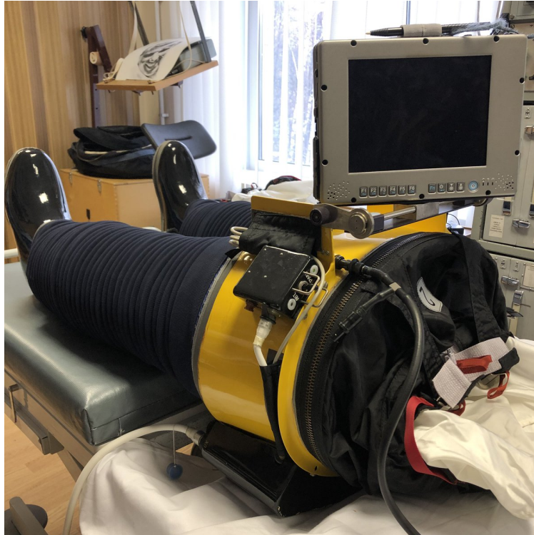
Figure 2.8: Chibis-M lower body negative pressure (LBNP) device. Image credit: NASA.
