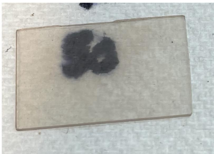
Figure III-13. (a) Reaction scheme to produce films of III-6 and UV-vis with III-6 and III-6-III-1 overlaid. (b) Optical photograph of film of Ru 2 BTC 4 Cl after 50 bilayers.
