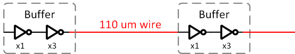
Figure 7.26: Inverter-based clock buffer.
