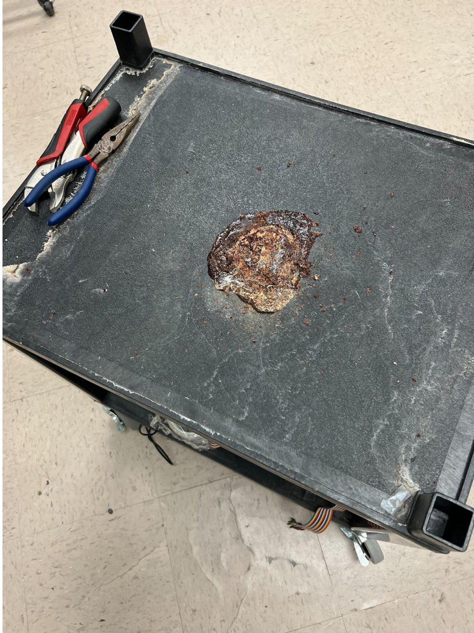
Figure 8. Melted Polycarbonate on the Cart that Held the Environmental Chamber
