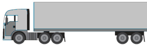
Figure 6.2 Selected axle configuration of autonomous truck (vehicle class 14).
