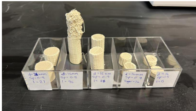
Figure 12: Layer height limitations results
