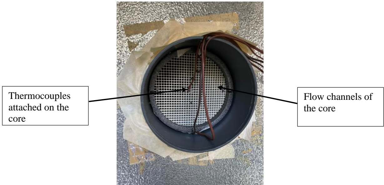
Figure 2.5: FBR core on the chamber side, along with thermocouples attached at the centre, top and the bottom.
