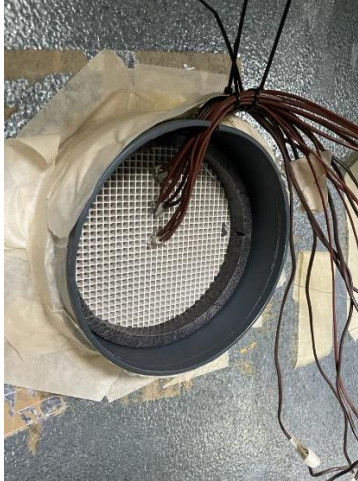
Figure 4.2: FBR core from the chamber side with thermocouples attached at 16 points
