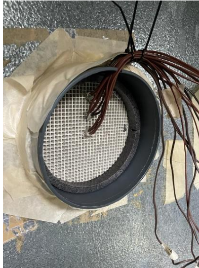
Figure 2.7: FBR core from the chamber side with thermocouples attached at 16 points
