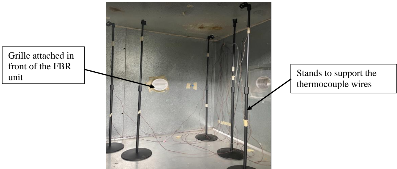
Figure 2.2: Inside of the FBR chamber, with thermocouples installed on the stands to measure chamber temperature and the FBR unit behind the white-colored grille.
