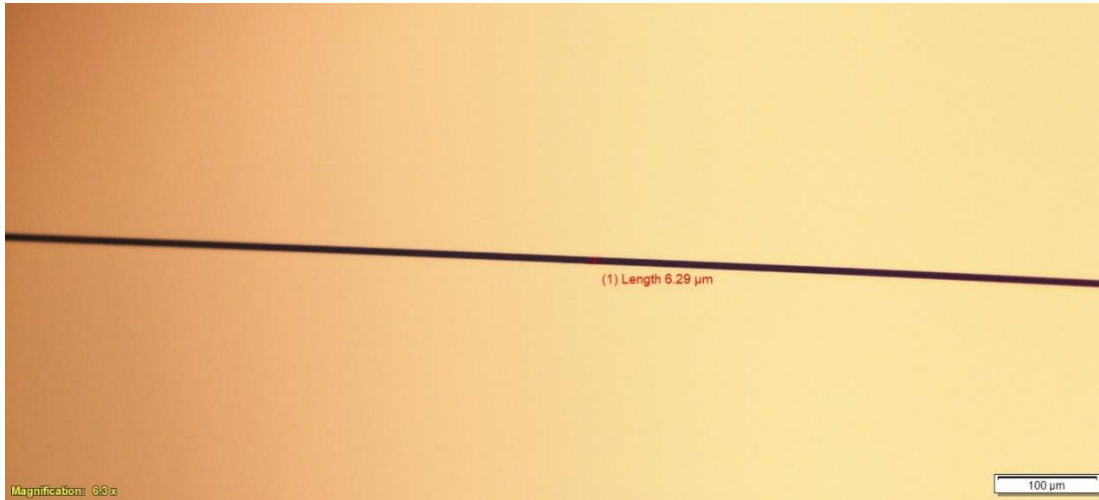
Figure A6: Optical microscopy image of T700 to measure its radius.
