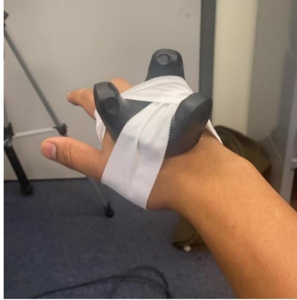
Figure 34. VIVE Tracker 3.0 secured to the dorsal side of the hand via athletic tape for virtual prosthesis position tracking
