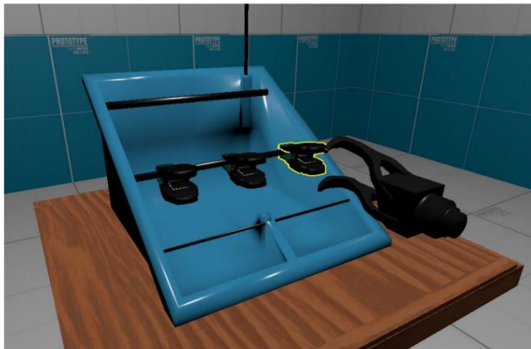
Figure 37. Highlighted outline of virtual clothespin. Serves as a visual cue to alert user of proximity to interactable object
