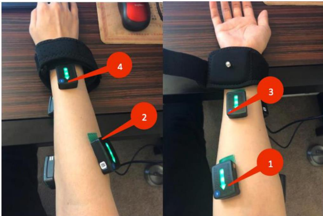
Figure 35. EMG sensor placement on flexor carpi radialis (1), extensor carpi radialis longus (2), flexor digitorum (3), and extensor digitorum (4)
