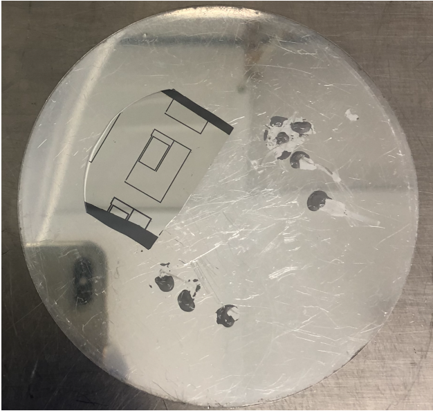
Figure 2.11: To prepare our sample for etching, it needs to be placed onto a carrier wafer. Heat sink paste (shown as dots above) is used to promote anisotropy through thermal conductivity and mount the sample to the carrier wafer so it does not move.
