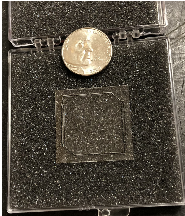
Figure 3.6: A fully fabricated fused silica pendulum resonator. This model used an earlier design where the flexures thinned out toward the ends. The experimental fundamental frequency for this model was roughly 32 Hz and the Q measurement in air was roughly 2,035.
