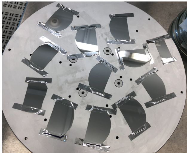
Figure 2.8: The silicon pieces are coated with a layer of aluminum. The aluminum acts as a selective hard mask for the remainder of the fabrication process. This aluminum can be easily removed after fabrication using an aluminum etchant.
