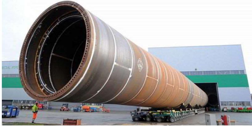
Figure 1.3 Monopile of 7.8 diameter used in Veja Mate offshore wind facility. Reprinted from (Skopljak 2016)
