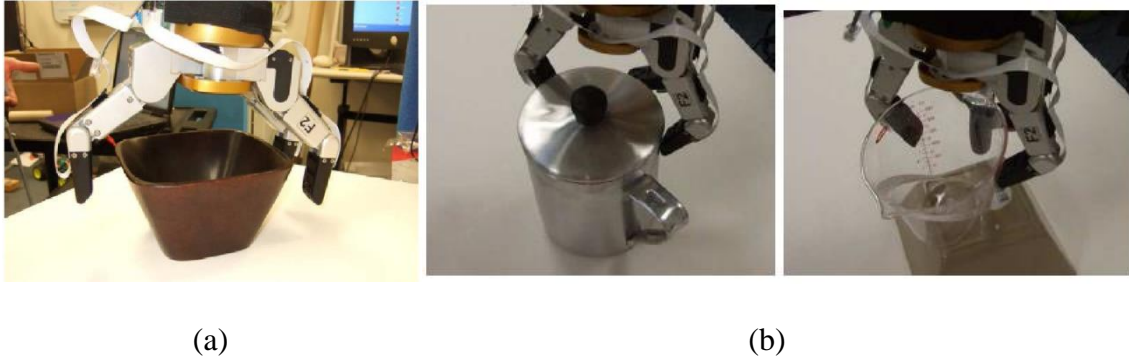
Fig. 2. 7. Optical proximity sensors for robotic grasping. (a) Three-fingered Barrett Hand with optical proximity sensors mounted on the fingertips. (b) Failure cases with a shiny can and a transparent cup. Reprinted with permission from [17] © IEEE.
