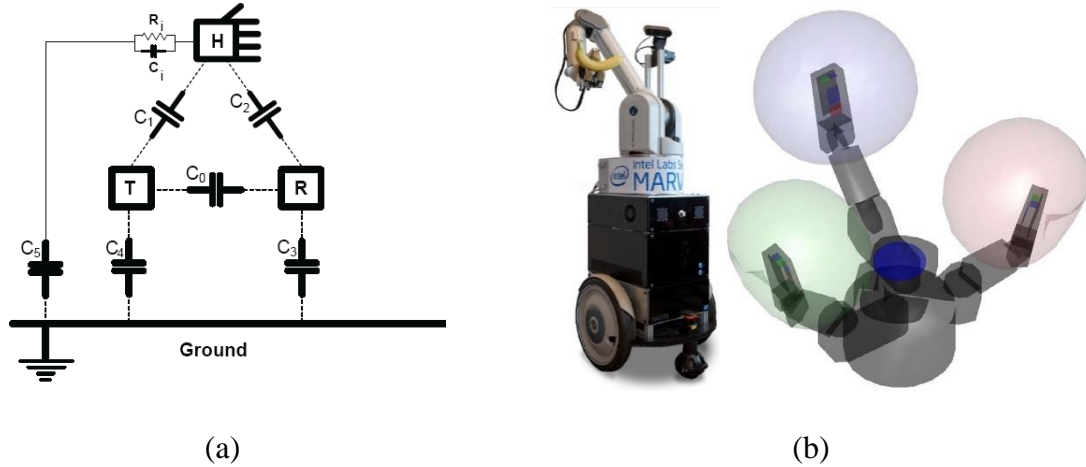
Fig. 2. 6. Electric-field near-distance sensors for robotic grasping. (a) Lumped circuit model for electric-field sensing of a hand. Reprinted with permission from [13] © IEEE. (b) Photograph of mobile manipulation platform, with electric-field pretouch-enabled hand. Reprinted with permission from [15] © IEEE.
