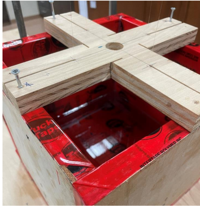
Figure 2.23. Close up view of fiber placements in the slots of the fiber positioner.
