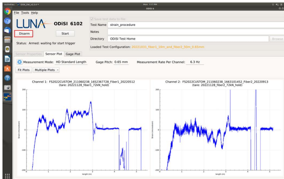
Figure 2.49 Disarm the system from acquiring data.
