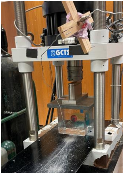
Figure 2.53 Sample in load cell oriented for injection test (shield is not pictured for clarity of set up).
