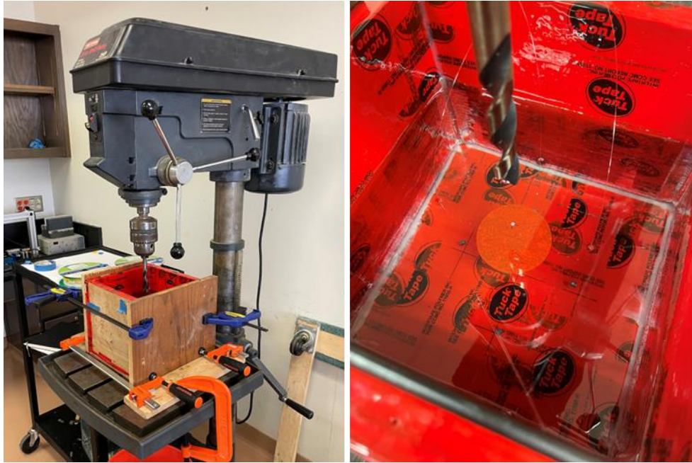
Figure 2.27. Mill press set up used to drill the hole for the injection tubing.
