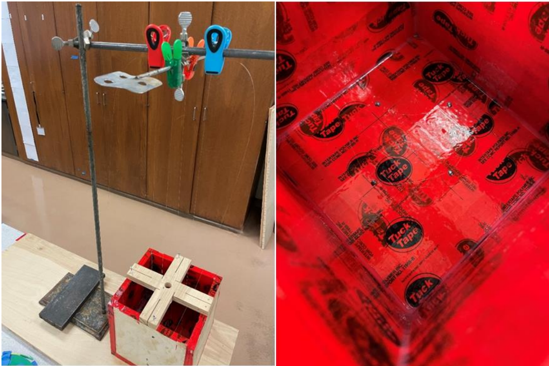
Figure 2.22 Distributed strain sensor suspended over the epoxy mold through the fiber positioner (left). Fishing weights hang slightly above the bottom of the epoxy mold two inches offset from the center (right).
