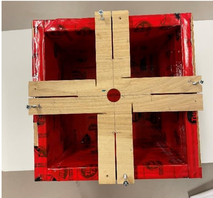
Figure 2.16 Fiber positioner centered and anchored to top of epoxy mold.
