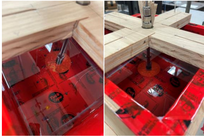
Figure 2.28. Injection tubing before (left) and after (right) layer four is poured.
