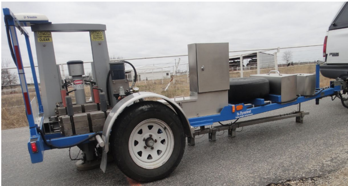
Figure 6. Falling Weight Deflectometer. Reprinted from [28].
