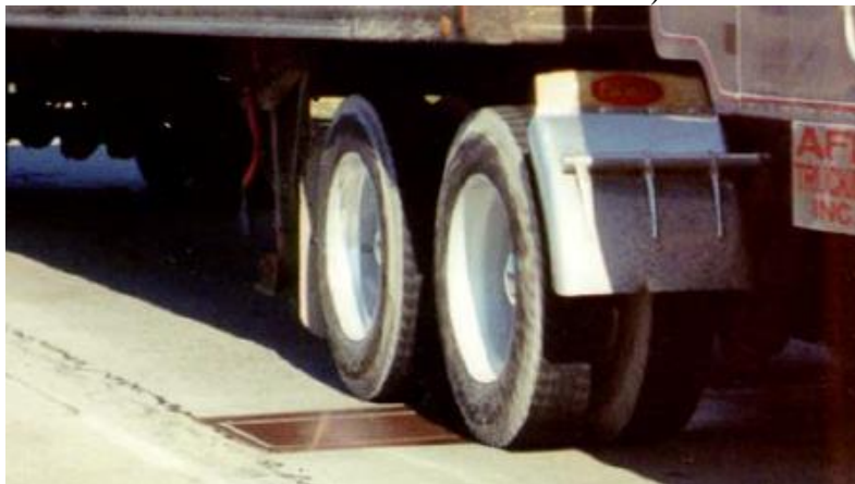
(b) Bending Plate WIM Scale Used for Vehicle Weighing (reprinted from VPG 2011)
