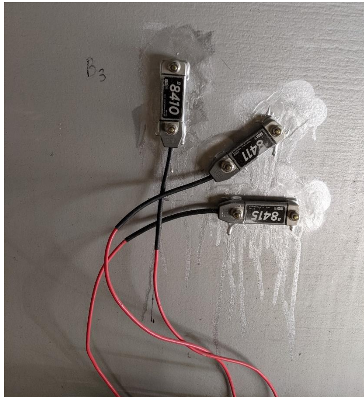
Figure 5.29. Strain Rosette at North End (Bridge #3).
