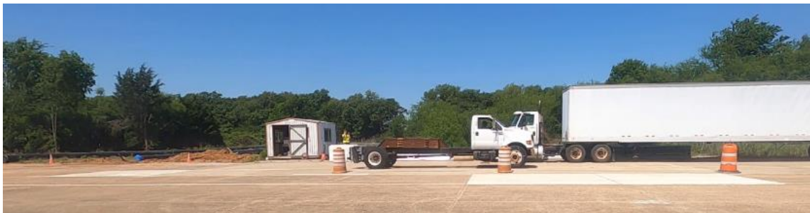
(b) Two Vehicles Reached Midspan of the RELLIS Bridge from Opposite Directions
