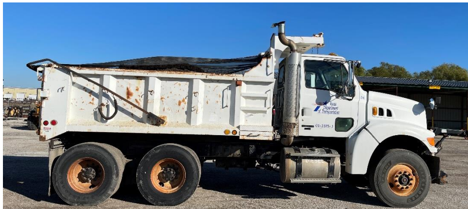
Figure 5.36. Calibration Truck A for Bridge #3.
