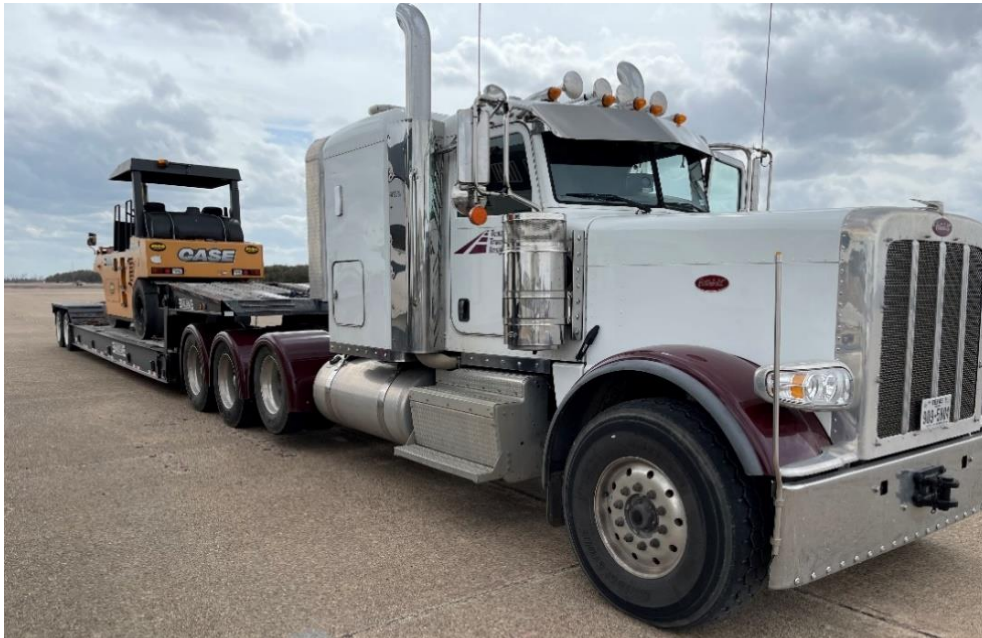
Figure 5.8. TTI Tractor-Trailer Loaded with a Roller Compactor.
