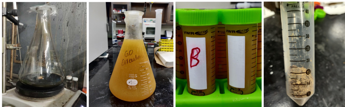
Figure A.1: Stages involved in the synthesis of GO (a) Reaction of graphite, sulfuric acid, and potassium permanganate mixture (oxidation), (b) Mixture post-hydrogen peroxide addition (oxidation arrested), (c) Graphene oxide washing (centrifugation), (d) Final product after complete drying in a vacuum oven.
