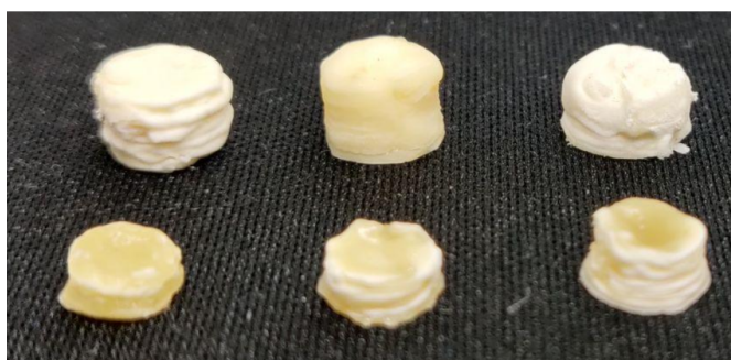
Figure 3.5: Printed structures salt removed post annealing (top) compared to printed structures annealed post-salt removal (bottom)
