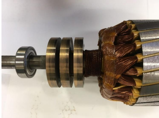
Fig. 57. Sliprings Installed on the Inner Rotor
