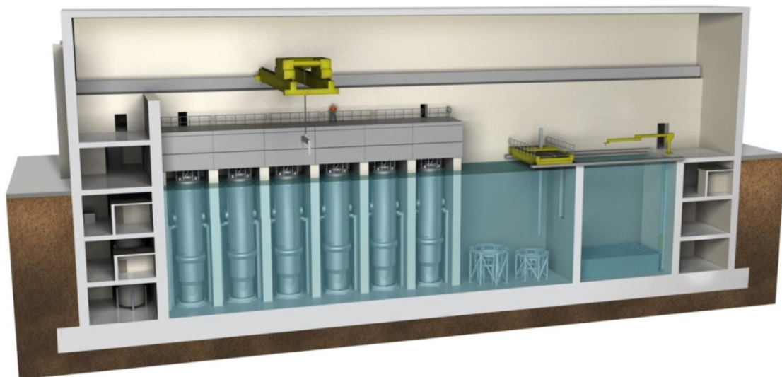
Figure 1. SMR configuration of NuScale Power Module developed by NuScale Power Inc., United States of America. Reprinted from [4]
